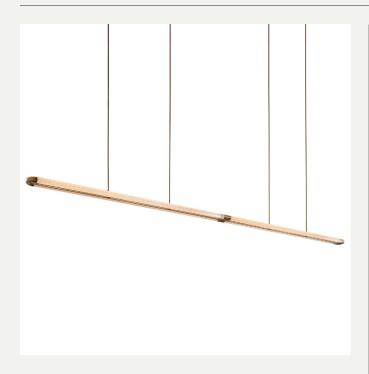
LIGHT SOURCE: MATERIALS: LINEAR 24V LED MODULE / 2700K BRASS, GLASS 90W / 11050 LUMENS WEIGHT: 26 KG (APPROX) DIMMING: PHASE (MAINS) DIMMING USING SUPPLIED 2 X 24V DRIVER OPTIONAL ACCESSORIES: DALI DRIVER 0-10V DRIVER VOLTAGE: 24V D.C (DRIVER LOCATED IN EACH CEILING CANOPY) SUSPENSION: DROP ROD AT 100MM INCREMENTS CERTIFICATIONS:
